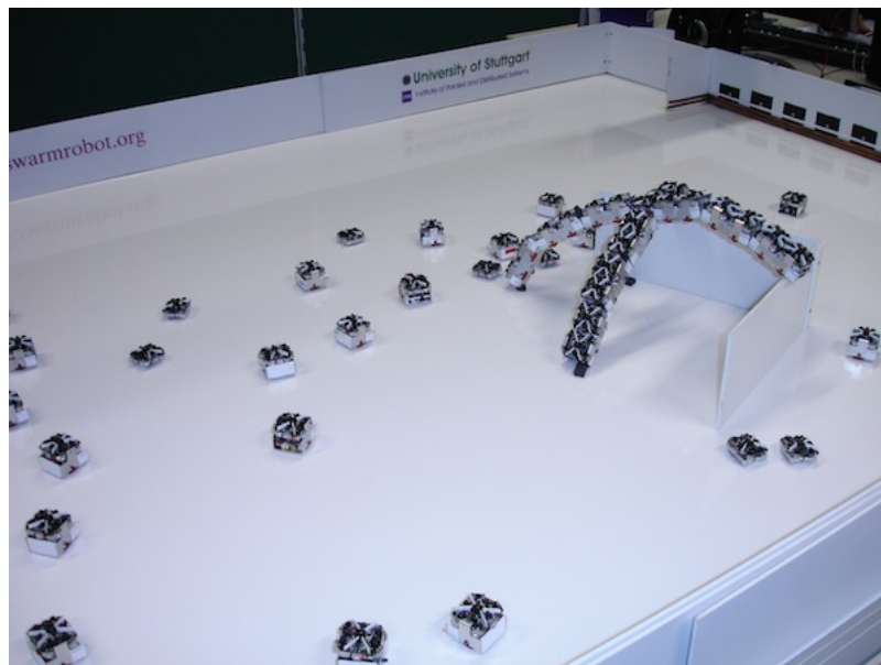
Figure 3.3: Several swarm robots self-assembled to overcome an obstacle in the arena [Sym].
