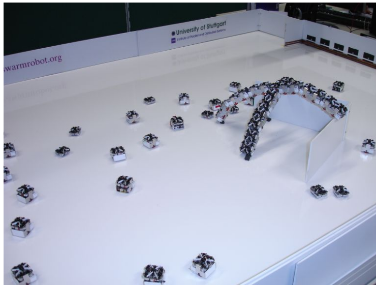
Figure 1.2: Multi-Robot-Organism climbing an obstacle
