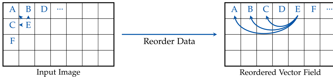
Figure 4.8: Schematic drawing of the reordered data of the vector field. The letters mark the position of the block in both arrays and the arrows show the dependencies of block E.
