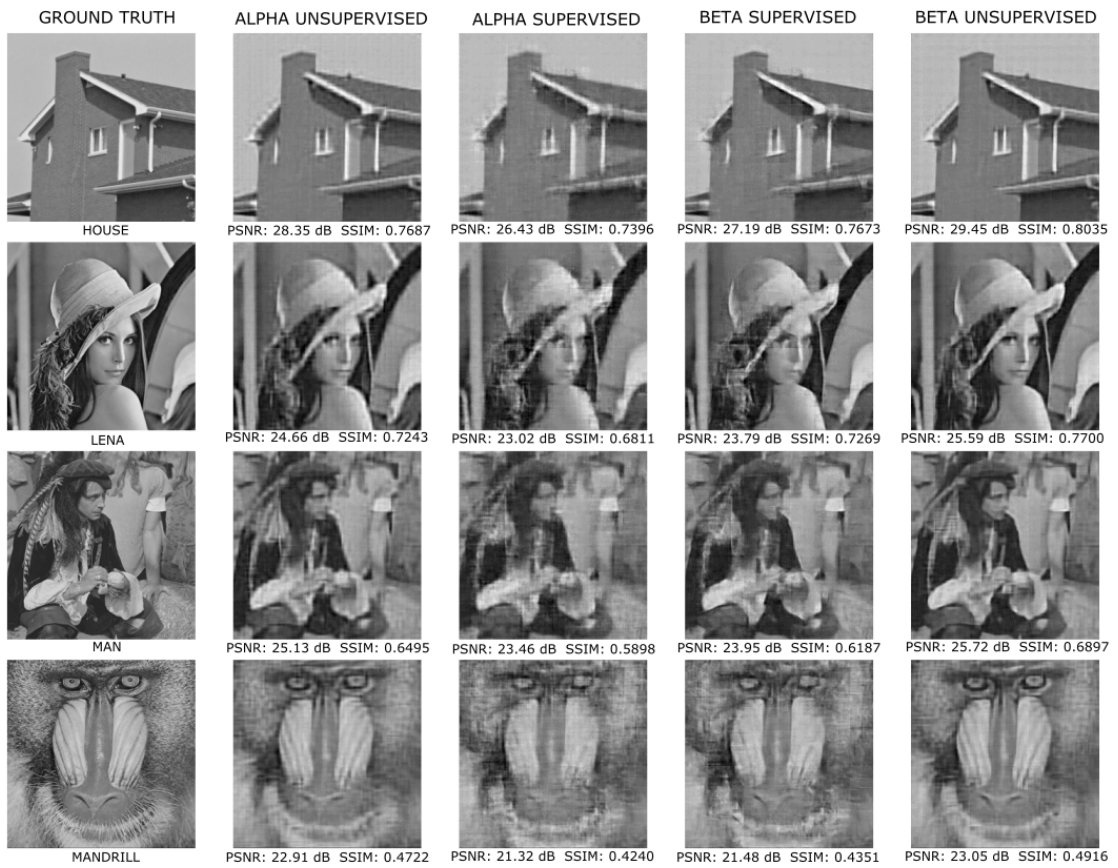
Figure 4.11 – Reconstructed house, lena, man and mandrill images compared against the ground truth, PSNR and SSIM.
